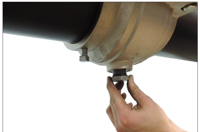
3. REMOVE PLUG: Using a 1\frac{1}{4} " wrench (for the 3 to 8" valves) or a 1\frac{1}{2} " wrench (for the 10 to 12" valves), remove the plug from the bottom of the valve body.
