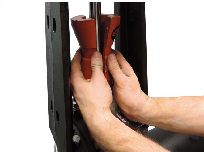
2c. Remove the T-bolt clamp and split the two halves of the shaft collar to remove.
