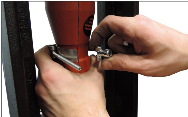
2b. Using a \frac{7}{16} " deep-well socket wrench, remove the nut on the T-bolt clamp and pull the clamp apart.
