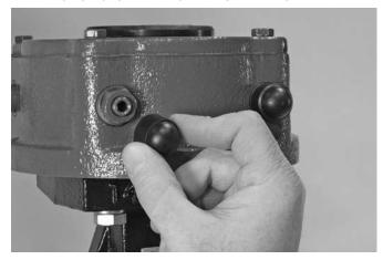
1. Remove the dust cap from the left side of the gear operator.
