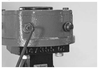
Using the allen wrench, tighten the internal set screw (clockwise) until it contacts the internal quadrant gear.
