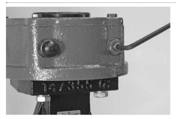
5. Using the allen wrench, tighten the internal set screw (clockwise) until it contacts the internal quadrant gear.
