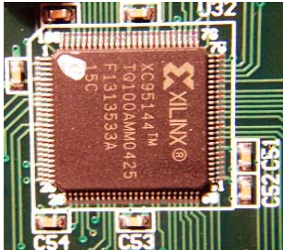
Figure 5 - No Corrosion Between Pins
