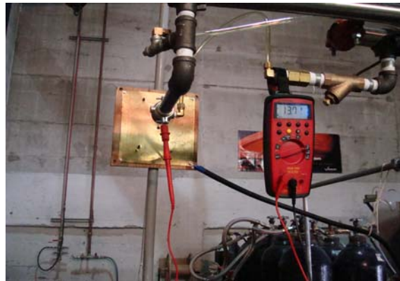
Figure 8 – Emitter discharge set up with copper plate
