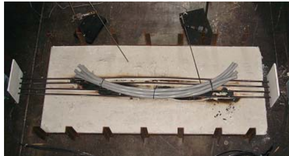
Figure 1 - Cable Bundle-Post Fire
