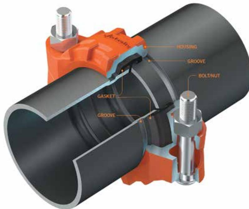
There are several attributes of the mechanical joint assembly that make it resistant to extreme heat: the ductile iron housings; the gasket material properties and the resulting sealing force when the bolts and nuts are fully assembled.
